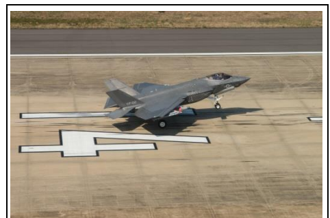
PHOTO: CF-2 completed the final SDD flight at Naval Air Station Patuxent River, Md., 11 April 2018. The F-35C completed a mission to collect loads data while carrying external 2,000-pound GBU-31 Joint Direct Attack Munitions (JDAM) and AIM-9X Sidewinder heat-seeking missiles.
