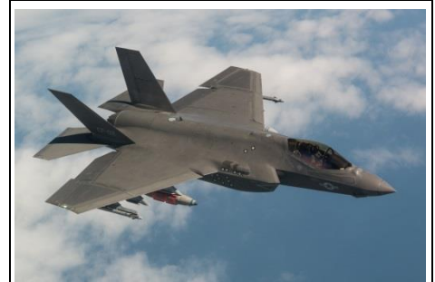
PHOTO: The final SDD Test flight CF-2 Flt 596 was piloted by BAE Test pilot Mr Peter Wilson, 11 April 2018. The F-35C completed a mission to collect loads data while carrying external 2,000-pound GBU-31 Joint Direct Attack Munitions (JDAM) and AIM-9X Sidewinder heat-seeking missiles.
