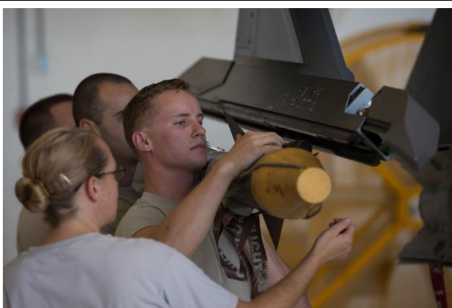
Airmen from the 33th Aircraft Maintenance Squadron load an AIM-9X missile on to an F-35A's external weapons pylon July 20, 2016, at Eglin Air Force Base, Fla. This milestone was the first time an F-35A at Eglin AFB was loaded with internal and external weapons and will help develop weapons loading procedures for the F-35 program. (U.S. Air Force photo by Senior Airman Stormy Archer)
