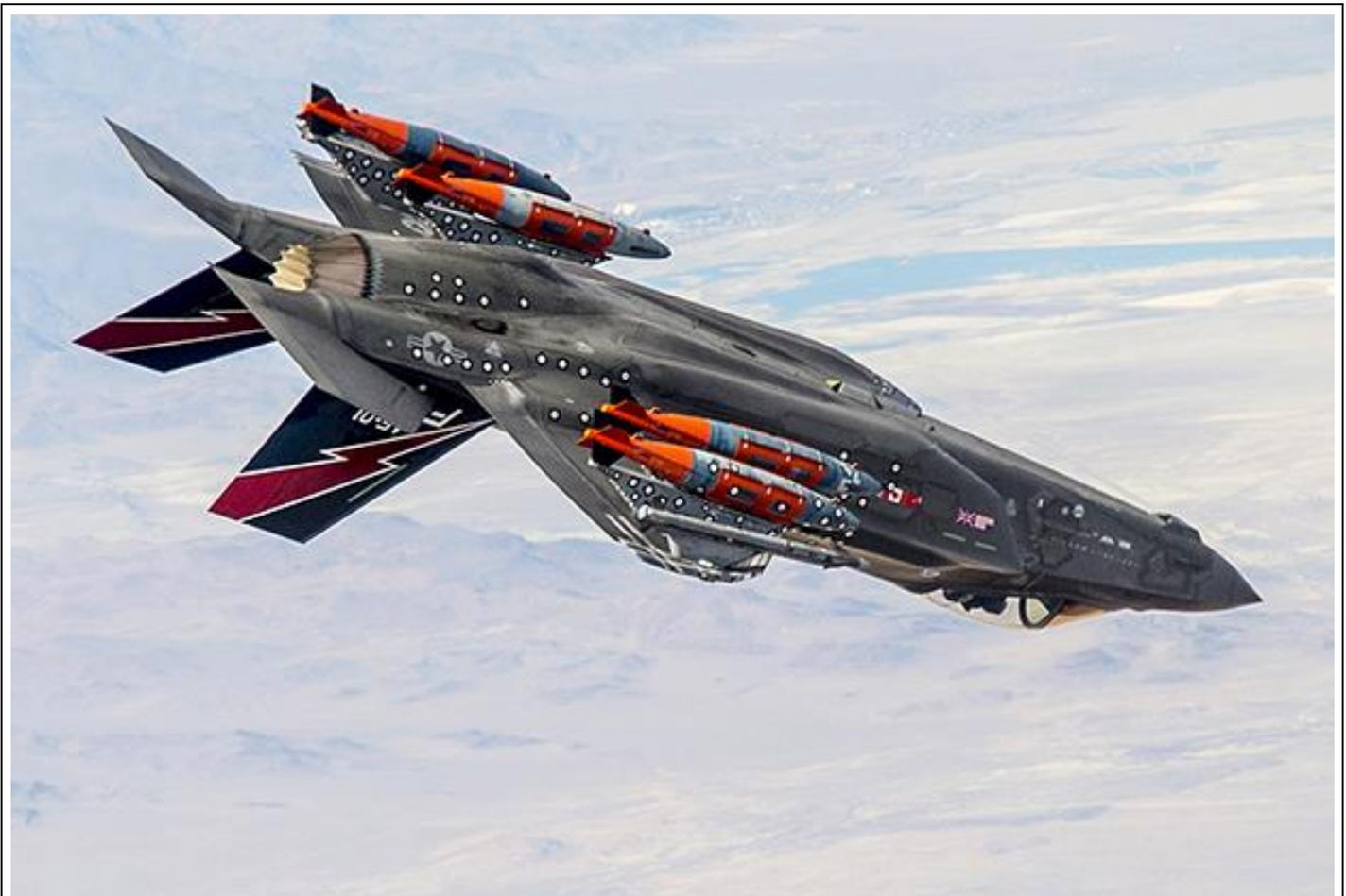
An F-35 in-flight over Edwards Air Force Base, Calif. The colorful markings on the bombs and the "spots" help calibrate cameras recording this flutter test. Photo by Darin Russell
