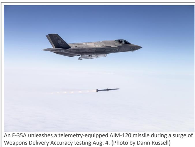
An F-35A unleashes a telemetry-equipped AIM-120 missile during a surge of Weapons Delivery Accuracy testing Aug. 4. (Photo by Darin Russell)
