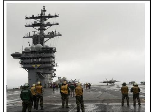
151002-D-AW822-459 ATLANTIC OCEAN (Oct. 2, 2015) - An F-35C Lightning II carrier variant Joint Strike Fighter from the Pax River Integrated Test Force conducts its first arrested landing aboard the aircraft carrier USS Dwight D. Eisenhower (CVN 69). Two F-35Cs from the Salty Dogs of Air Test and Evaluation Squadron (VX) 23 are conducting follow-on developmental test (DT-II) sea trials aboard the Eisenhower. (Lockheed Martin photo by Andy Wolfe.)
