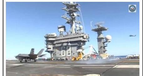
An F-35C Lightning II carrier variant joint strike fighter conducts its first arrested landing aboard the aircraft carrier USS Nimitz (CVN 68). Nimitz is underway conducting routine training exercises. (U.S. Navy photo by Mass Communication Specialist 3rd Class Kelly M. Agee/Released)
