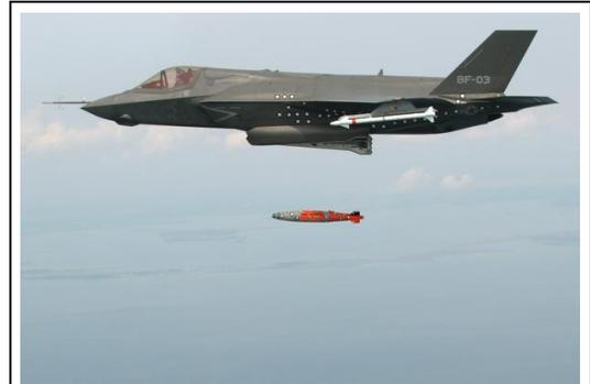
F-35B test aircraft BF-3, flown by Lockheed Martin test pilot Dan Levin, completed the first aerial weapons release Aug. 8, for any variant of the aircraft. BF-3 dropped an inert 1,000-pound GBU-32 Joint Direct Attack Munition over an Atlantic test range from an internal weapons bay. (Photo courtesy of Lockheed Martin)
