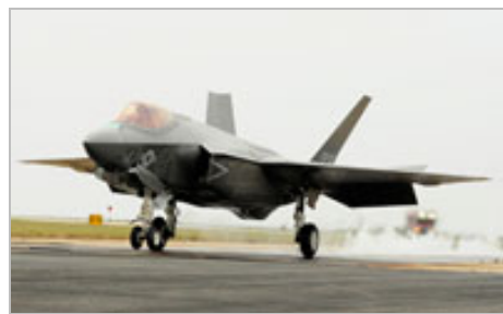
Navy test pilot Lt. Chris Tabert flies F-35C test aircraft CF-3 off the TC-7 steam catapult at NAS Patuxent River Nov. 4. (U.S. Navy photo)
